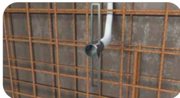
Fasten grommet with wings directly to the steel reinforcement or nail with the base to the formwork. Simply open with a screwdriver after concreting.
